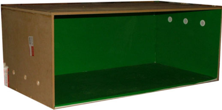
Cage with Contact Covering (Note: the vents are already cut and installed on this cage)
