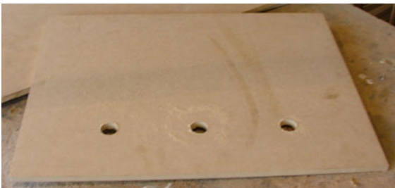
Round drill holes - these are 1 1/8" diameter. and suit cupboard vents.
